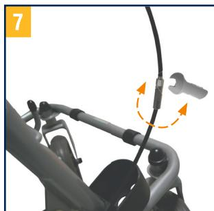
For desired braking strength adjust the brake either manually at the screw on the housing of the brake (picture 6) or with the suitable tool (not included) on the brake wire (picture 7).
