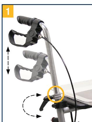
Insert the tube of the adjustable handgrip into the frame at least to the "MAX" marking.
